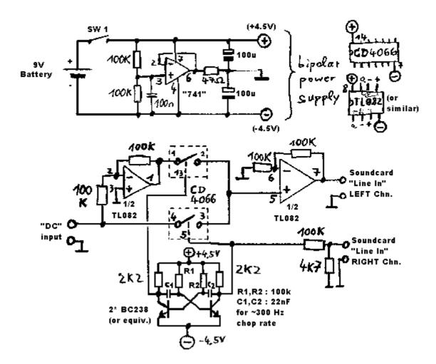
A signal with a few hundred millivolts may be fed into the "DC input", either polarity. Note that the analog switch is not connected to ground, but to a positive and negative power supply. The same applies to the double OPAMP, like the TL082 used here. If you don't need battery-powered operation, leave the circuit around the "741" OPAMP away and use a simple dual power supply instead (+/- 5 V).
